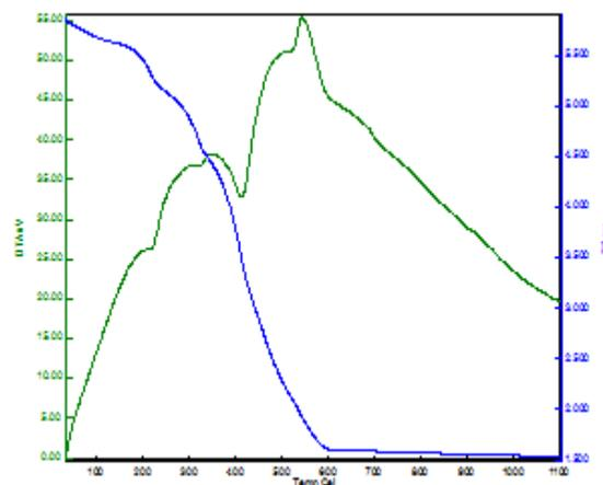
Fig 3. TGA-DTA of Cr<sub>2</sub>O<sub>3</sub>
