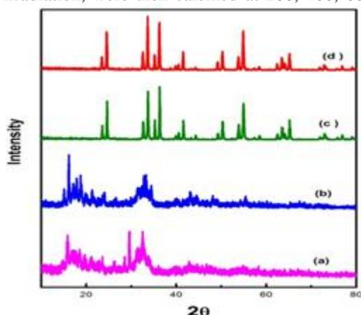
Fig 1. Powdered XRD pattern of the as prepared and the calcined  $\text{Cr}_2\text{O}_3$  at 200, 400, 600 and 800°C .
