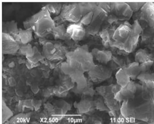
Fig 2. Sem image of Cr<sub>2</sub>O<sub>3</sub>
