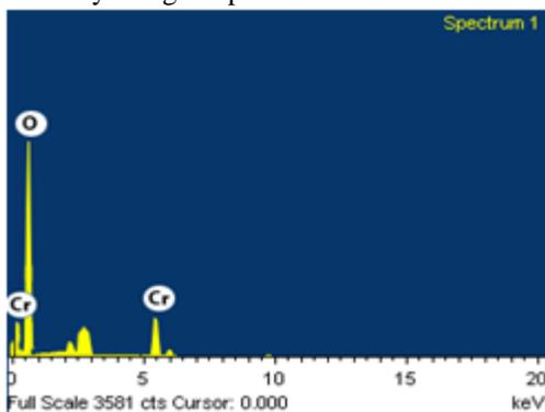
Fig 4. EDAX spectra of Cr<sub>2</sub>O<sub>3</sub>
